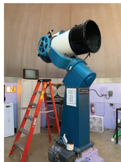
The 16-inch Celestron Schmidt Cassegrain telescope in the current Laws Observatory atop the Physics Building.
